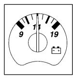
When the engine is running, the gage shows the condition of the charging system. Readings between the low and high warning zones indicate the normal operating range.
